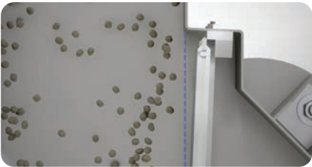
Recessed blade(s) to protect the blade(s) & seal(s) from abrasion
