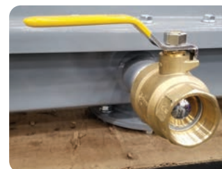
Inlet ports with ball valves to adjust the amount of air being injected into the air-gravity conveying system. Each section of the conveyor has inlet ports, located along the side of the lower air chamber.
