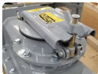
Cleanout ports to inspect for product in the lower air chamber and maintain, if necessary. Each section of the conveyor has a cleanout port, located along the bottom of the lower air chamber.
