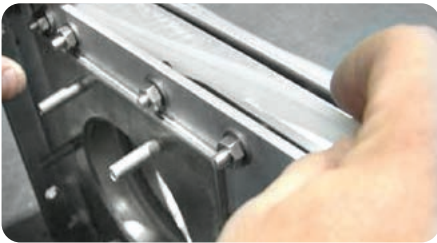
Shimming system for in-line maintenance
