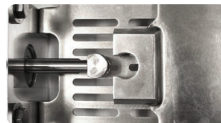
Specially designed clevis allows for quick blade removal
