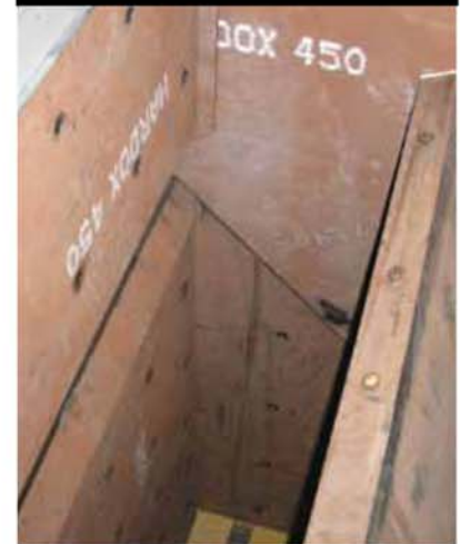
Figure 8: abrasion-resistant liners ensure that materials abrade upon highly-durable, replaceable parts rather than abrading upon the diverter itself
